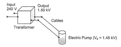
a) Calculate the number of turns required on the primary winding of the transformer.
