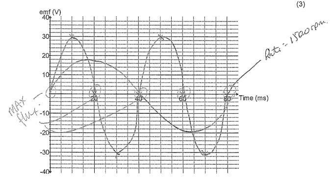
e) Identify three times on the graph when the flux enclosed by the coil is a maximum value at 1500 rpm. Circle these times.
