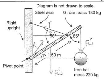
a. Identify all the forces acting on the girder by drawing them on the diagram.
