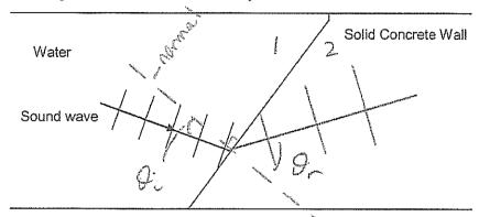
a) Draw a possible path of the sound wave as it refracts into the concrete. Indicate appropriate angles. Shows refraction away from normal Or) Di
